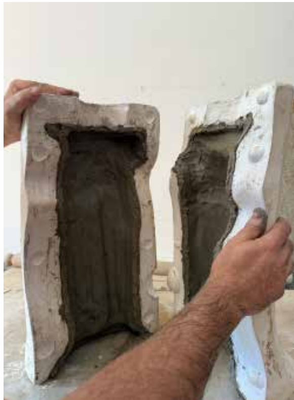
Joining of two halves of the press-moulded lower part of Minerva
