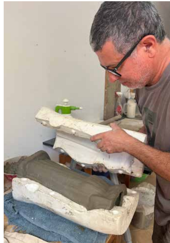
Removing the upper part of the press-moulded lower part of Minerva from the plaster mould
